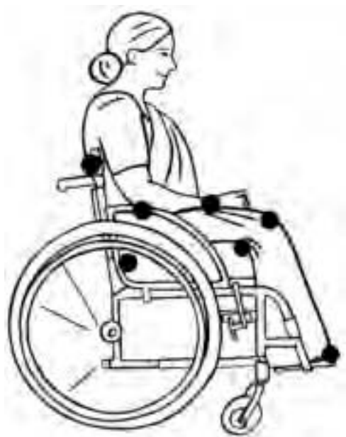
Fig. 2.5. Common pressure sensitive areas (side view)
